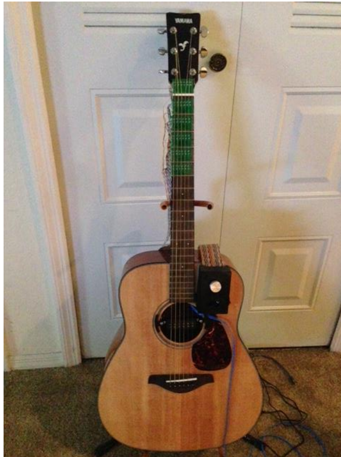
Figure 55 – First Hex Pickup Prototype
