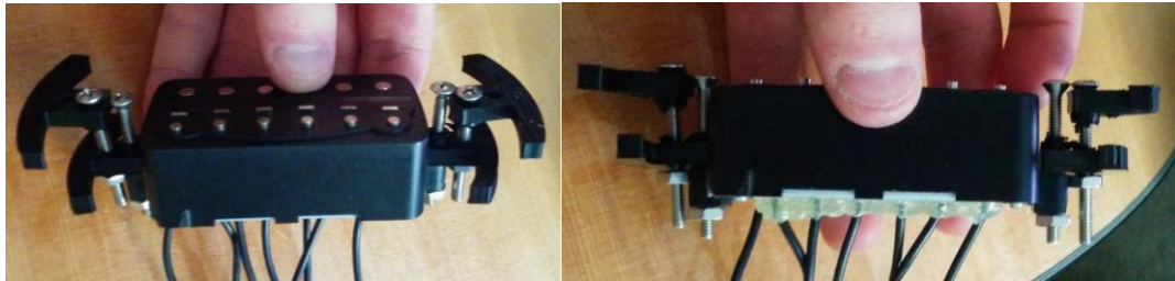
Figure 52 – Clamping Mechanism for pickup
