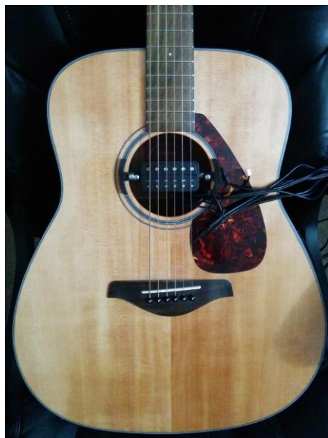
Figure 54 – Hex Pickup with custom clamps
