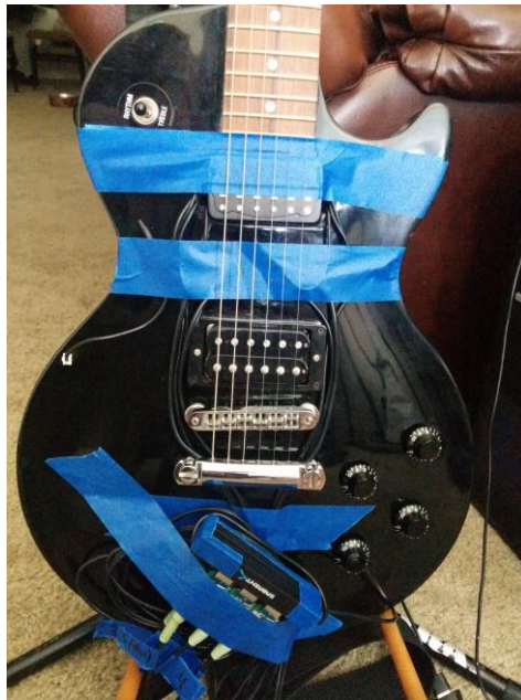
Figure 53 – First Hex Pickup Prototype
